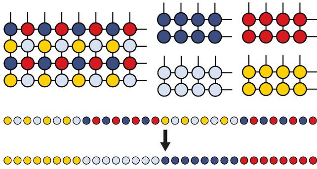
**Fig. 6.** Left: a SPGrid block of  $4 \times 8$  in which the nodes are ordered lexicographically, Right: the transposed colored storage enables efficient vectorization for Gauss-Seidel iteration. Bottom: Transposition operation of a SPGrid block illustrated in a linear memory layout.
