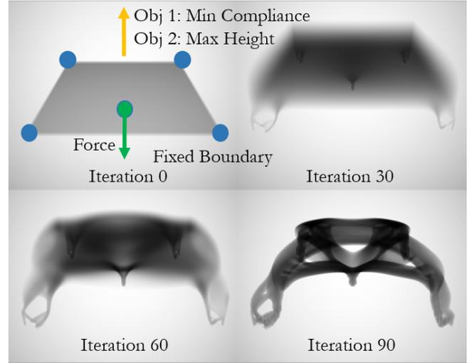
**Fig. 8.** Unbounded topology optimization for a quadpod structure. A thin membrane is initialized (a), evolved upwards (b), and converge to a clear structure (c and d), guided by a combined objective of both minimum compliance and maximum height.
