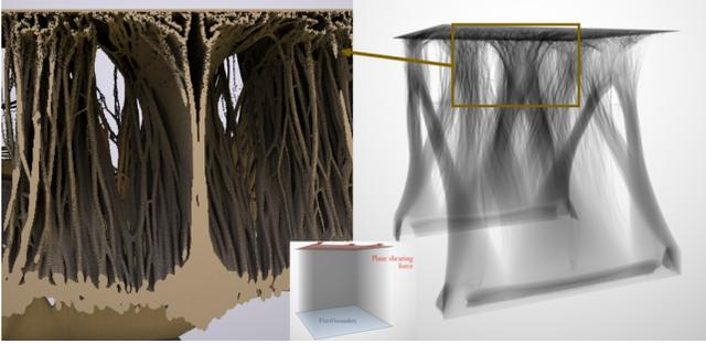
**Fig. 13.** Optimized structures supporting a plate to resist horizontal shear forces are generated at a resolution of  $640 \times 640 \times 640$ . The left figure is a cross-section of the structure exhibiting various filamentary features. The right picture shows the volumetric rendering. The sub-image in the middle shows the boundary conditions, including a fixed boundary and a shear force on the bottom and top plane in separate.
