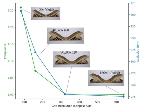
**Fig. 12.** Relation between the grid resolution, the optimized structural compliance, and the level of details (measured by the sum of  $L_2$  norm of the density's Laplacian). The plot shows that the high-resolution simulation enables detailed structures with low compliance.
