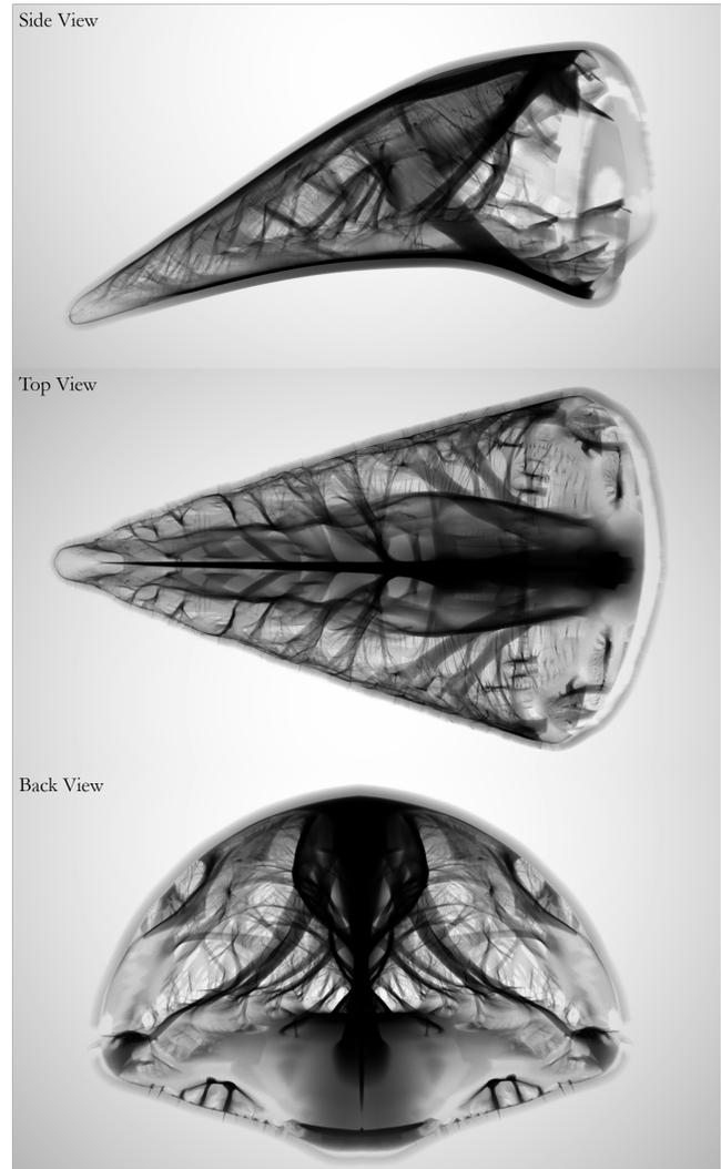
**Fig. 1.** The interior structures supporting the shell of a bird beak generated using our narrow-band topology optimization algorithm with  $k1, 040, 875, 347$  (1.04 billion) active FEM voxels. The resolution of the background grid is  $3000 \times 2400 \times 1600$ . The three figures show the volumetric rendering of the same structure from different views.
