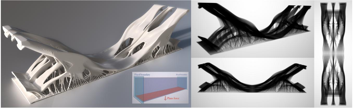
**Fig. 3.** An optimized bridge structure is obtained on a  $271 \times 540 \times 1081$  grid (157 M voxels) with mirror boundary conditions applied on the  $X$  and  $Z$  axes. The left figure shows a solid render, and the right three figures show the visualization of the density field from different camera views. The middle sub-image illustrates the boundary conditions, including fixed boundaries on the sides and a load applied on the bottom plane.
