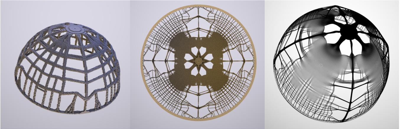
**Fig. 2.** Structures with codimensional thin features are obtained by running the narrow-band algorithm on a thin hemispherical shell. The boundary conditions include a fixed boundary on the top and an external load applied on the cross surface on the bottom. As the grid resolution increases from  $512^3$  (left) to  $2048^3$  (right), thin-shell structures are observed to dominate, matching the tendency studied in [Sigmund et al. 2016].
