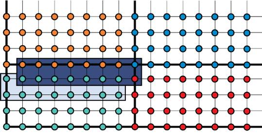
**Fig. 4.** The offset passed to VectorGet points to an sequence of SPGrid entries with SIMD-width alignment (light blue box). Using a stencil offset, e.g., shifts the region to be loaded by VectorGet, as shown in the dark blue box. The data of this shifted box may originate in several distinct SPGrid blocks (indicated by different node colors).
