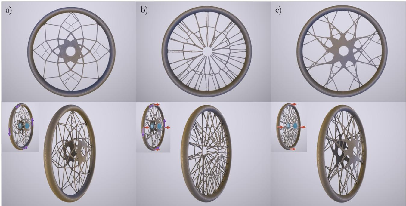
**Fig. 14.** Optimized wheel structures are generated using our algorithm. Structure (a) and (b) are obtained with in-plane tangential force boundary and out-of-plane normal force boundary. Structure (c) is optimized with a linear combination of objectives in both (a) and (b).
