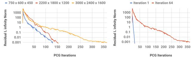
**Fig. 9.** (Left) Convergence comparison of the bird beak example of different resolutions at the last topology optimization iteration.<sup>†</sup> (Right) Convergence comparison of the one-billion-voxel bird beak example at different topology optimization iterations.
