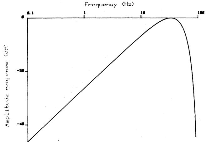
Fig. 4. Amplitude response of the digital derivative filter.
