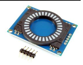
This board is equipped with a Circular LED Bar with 16 independent LEDs, each of which illuminates two segments of the bar, for a total of 32 segments, thanks to which you can make very eye-catching visual effects, and that will give an aesthetic touch to your projects.
