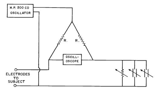
CIRCUIT FOR MEASUREMENT OF IMPEDANCE
