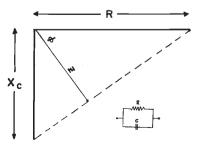
FIG. 5. Relationship of phase angle  $(\emptyset)$  and impedance (z) to resistance (R) and capacitance reactance (X<sub>c</sub>).
